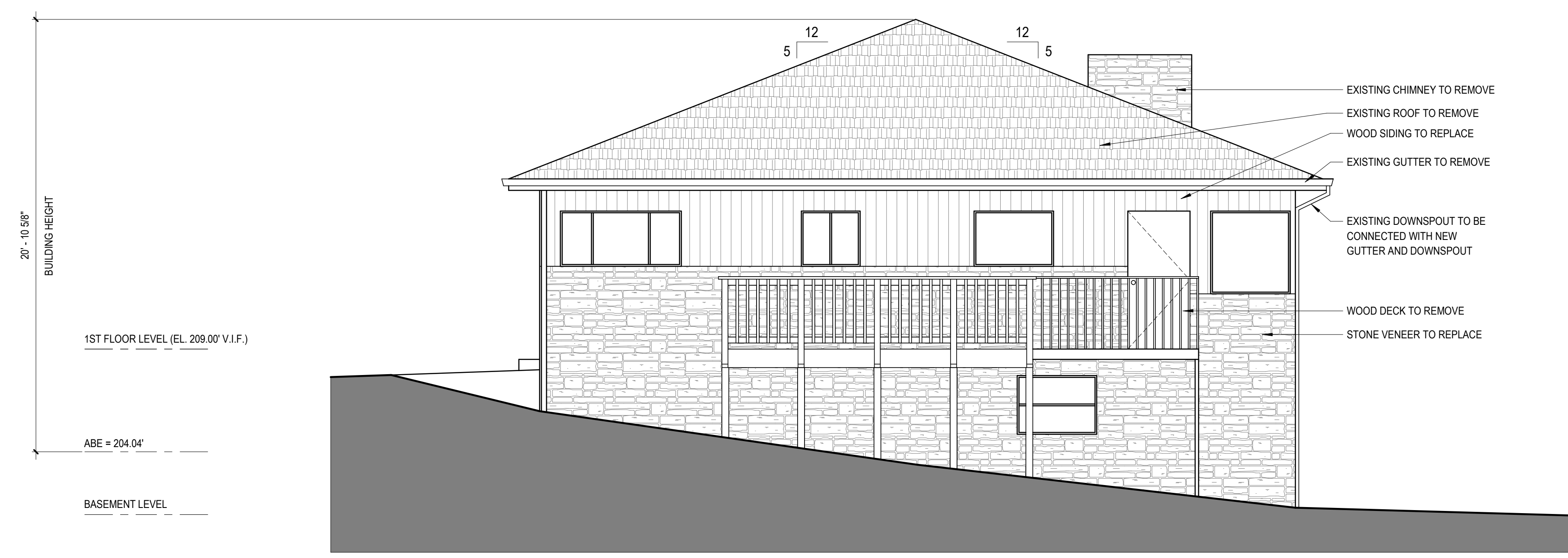
1 BUILDING ELEVATION EAST - EXISTING 1/4" = 1'-0"
